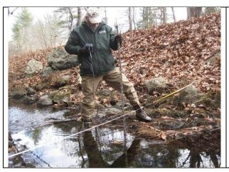
To determine stream flow, the entire width of the stream is assessed using a flow meter, located at the bottom of the hand-held stick. NHDES personnel must take multiple measurements to determine water height and flow at each depth. Several times each year, scientists record the various flows across the stream, the visual height on the white measuring stick, and the pressure differential to assure the reliability of automated data collection.
